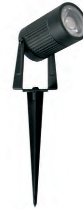
Model: HYL-5W-D17B Power: 5W Size: Φ50xW65xH310 Lumen: 360Lm IP65 Voltage: AC220-240V RA>80 CCT: 3000K/4000K/6500K PF>0.5 Beam angle: 30° Life span: ≥25000hrs Certification: CE
