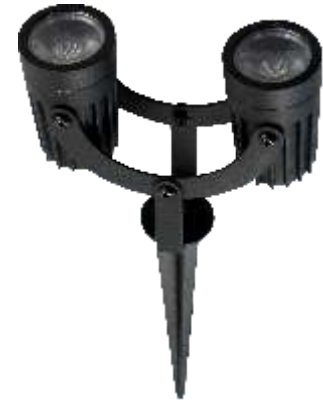
Model: HYL-3W-D17A Power: 3W Size: Φ40xW52xH240 Lumen: 200Lm IP66 Voltage: AC220-240V RA>80 CCT: 3000K/4000K/6500K PF>0.5 Beam angle: 38° Life span: ≥25000hrs Certification: CE
