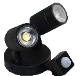
Model: HYL-5W-S17A-SE Power: 2*5W Size: Φ50xWΦ115xH150 Lumen: 2*360Lm IP44 Voltage: AC220-240V RA>80 CCT: 3000K/4000K/6500K PF>0.5 Beam angle: 30° Sensor angle: 120° Sensor distance: 0-8m Life span: ≥25000hrs Certification: CE
