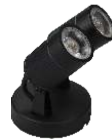
Model: HYL-5W-S17A Power: 2*5W Size: Φ50xWΦ115xH150 Lumen: 2*360Lm IP65 Voltage: AC220-240V RA>80 CCT: 3000K/4000K/6500K PF>0.5 Beam angle: 30° Life span: ≥25000hrs Certification: CE
