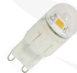
G9-103 Input Voltage(V): 220-240V Wattage: 1.8W Lumen: 120Lm Size: 16.9X41MM CCT: 2700-6500K Beam Angle: 360°
