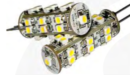
LED-G4-SMD A Input Voltage(V): DC8-30V Wattage: 1.5W 25PCS 3528 SMD Lumen: 80-100Lm Size: 10X45MM CCT: 2700-6500K
