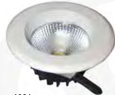
1031 Input Voltage(V): AC110/220V Wattage: 3W Lumen: 180-210Lm Size: Φ85X45MM Hole size: Φ65MM CCT: 2700-6500K Beam Angle: 45°
