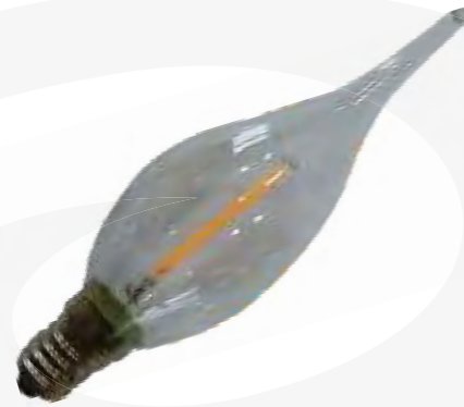
LE-202 Voltage:AC 220-240V Size (mm):35X120 Power :2W Lumen:200-220Lm Material:glass Color temperture:2700-6500K CRI >80
