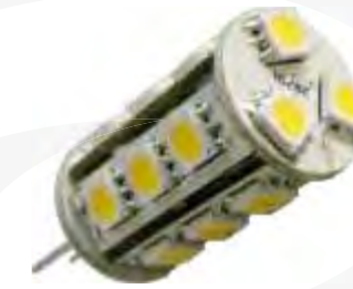
LED-G4-SMD B Input Voltage(V): DC8-30V Wattage: 3.6W 18PCS 5050 SMD Lumen: 160-200Lm Size: 18X33MM CCT: 2700-6500K
