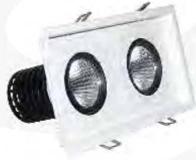
D104 Input Voltage(V): AC110/220V Wattage: 20W Lumen: 1400-1600Lm Size: 200X111X95MM Hole size: 198X98MM CCT: 2700-6500K Beam Angle: 23°
