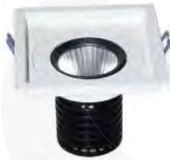
D102 Input Voltage(V): AC110/220V Wattage: 10W Lumen: 700-800Lm Size: 111X111X95MM Hole size: 98X98MM CCT: 2700-6500K Beam Angle: 23°
