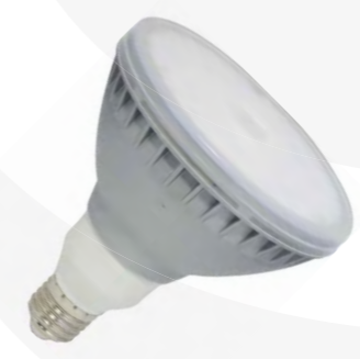
PAR38 Input Voltage(V): AC110/220V Wattage: 18W Lumen: 1150-1250Lm Size: 120X133MM CCT: 2700-6500K
