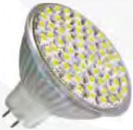
LED-MR16-3528 Input Voltage(V): DC12V Wattage: 3.5/4W 48/60PCS 3528 LED Bulb Lumen: 160/250Lm Size: 50X50MM CCT: 2700-6500K
