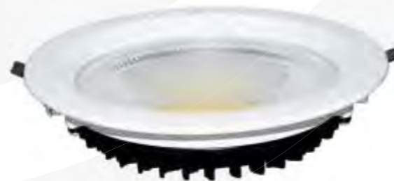
1036 Input Voltage(V): AC110/220V Wattage: 20W Lumen: 1200-1400Lm Size: Φ220X55MM Hole size: Φ198MM CCT: 2700-6500K Beam Angle: 85°
