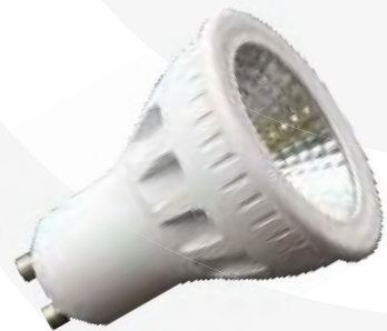
S030 Input Voltage(V):AC110-220V Wattage: 4W/6W Lumen: 300-320Lm/450-480Lm Size: 50X55MM/50X62MM CCT: 2700-6500K
