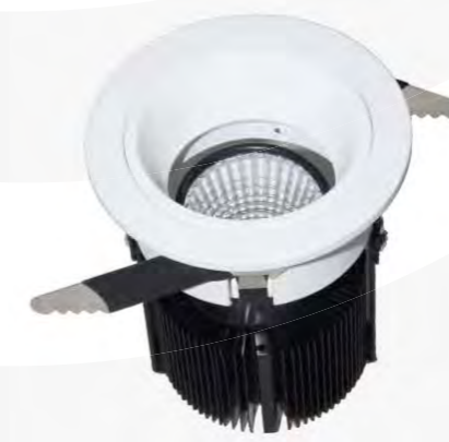
C310 Input Voltage(V): AC110/220V Wattage: 10W Lumen: 600Lm Size: Φ90X114MM Hole size: Φ78MM CCT: 2700-6500K Beam Angle: 21°
