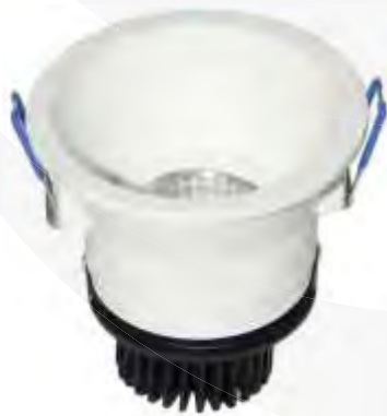
C406 Input Voltage(V): AC110/220V Wattage: 8W Lumen: 500Lm Size: Φ99X110MM Hole size: Φ92MM CCT: 2700-6500K Beam Angle: 19°
