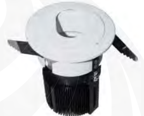
C306 Input Voltage(V): AC110/220V Wattage: 10W Lumen: 320Lm Size: Φ90X114MM Hole size: Φ78MM CCT: 2700-6500K Beam Angle: 29°
