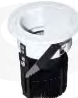
C304 Input Voltage(V): AC110/220V Wattage: 10W Lumen: 330Lm Size: Φ90X114MM Hole size: Φ78MM CCT: 2700-6500K Beam Angle: 29°
