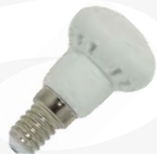
R50-02 Input Voltage(V): AC110/220V Wattage: 6W Lumen: 450-490Lm Size: 50X84MM CCT: 2700-6500K
