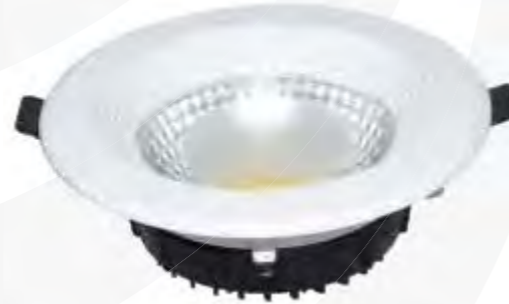
1034 Input Voltage(V): AC110/220V Wattage: 12W Lumen: 720-840Lm Size: Φ165X50MM Hole size: Φ138MM CCT: 2700-6500K Beam Angle: 65°
