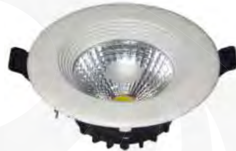
1032 Input Voltage(V): AC110/220V Wattage: 5W Lumen: 300-330Lm Size: Φ105X50MM Hole size: Φ85MM CCT: 2700-6500K Beam Angle: 45°
